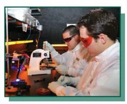
This team is testing resin curing lights to determine their ability to cure a variety of resinbased composites.
