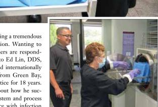
Wearing heavy-duty utility gloves, Nancy Figgins, the Central Sterilization Coordinator in the practice of Ed Lin, DDS, MS, wraps the clean and dry cassettes prior to sterilization. After the cassettes have been wrapped, Nancy loads them into the sterilizer. The cassettes are placed in a rack that allows adequate space for proper sterilization.
