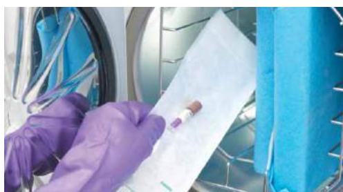
Assuming this strip is brown, after 10 minutes' cooling time has elapsed, both the test and the control vials are crushed and placed in the incubator for 24 hours. The operator can then view the color of the liquid in the test and the control vials – if the culture medium is still purple while the control test's culture medium is yellow, the test is negative, indicating sterilization occurred. If the color is yellow, the test is a fail (growth of spores has occurred during incubation).
